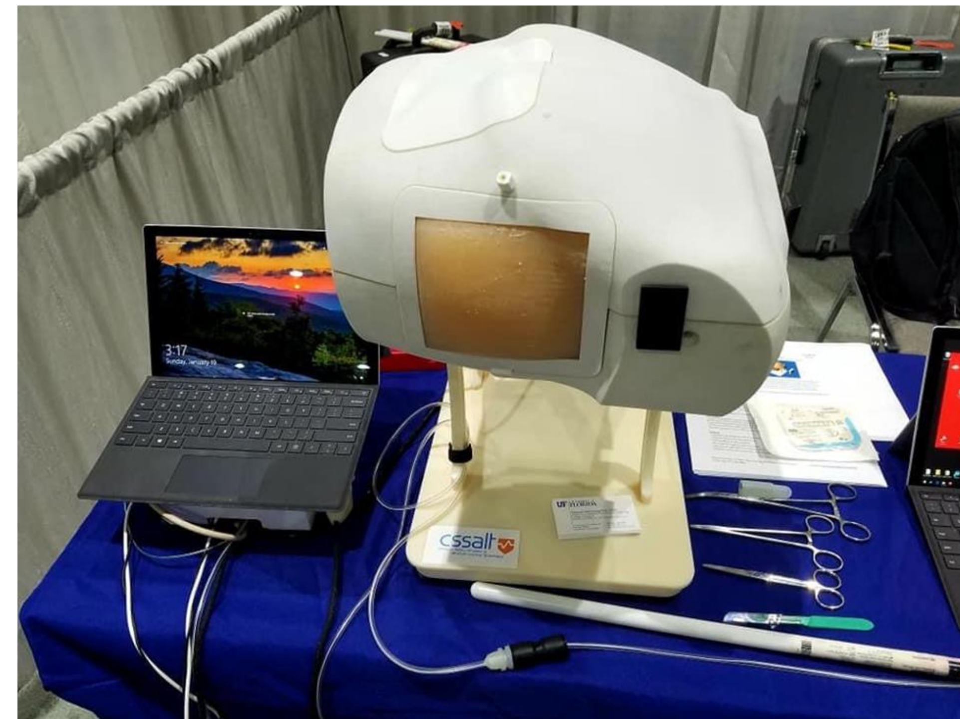
Figure 1: CSSALT mixed reality chest tube thoracostomy simulator.
