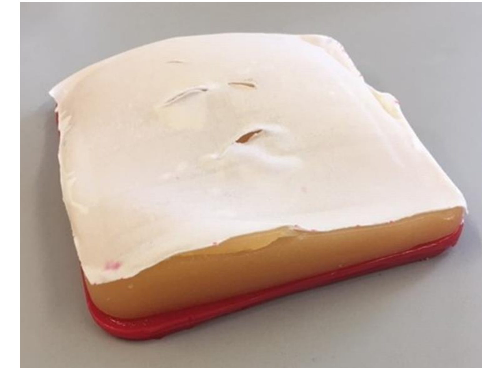
Figure 3: A used molded trilayer and durometer muscle/subcutaneous tissue/skin insert.
